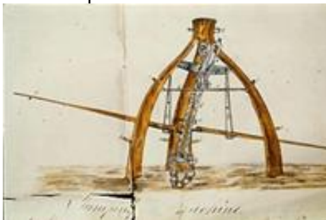
Lever Action Stump Puller
